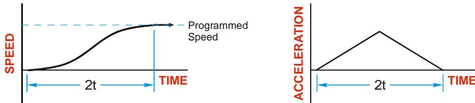
Figure 2.3 Triangular S-Curve Acceleration
