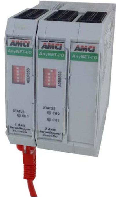
Figure 1.1 AnyNET-I/O Module Stack ANF1E (left) & ANF2 (right)
