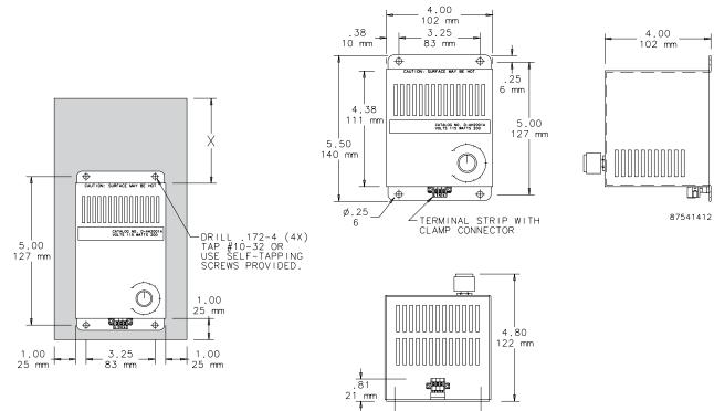
Dimensions and Clearance Range Drawing for DAH4001B, -2B and DAH8001B, -2B
